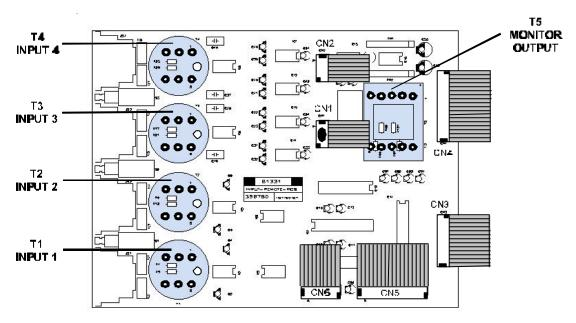
diagram 10 Printed board assembly 81331 showing the position of the input transformers NRS 90208
